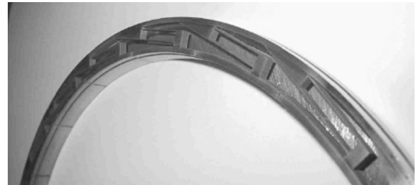
Fig. 62 Hydrodynamic brush seal (spring beam elements). 142
